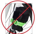
♠ WARNING: Untrimmed, excessive, or loose straps may stop the rotation of the wheel or release cargo, causing a loss of control and a crash that could lead to serious injury. Maintain at least 10mm clearance between wheels, fork, frame, or fender, and mounted cargo or straps.
